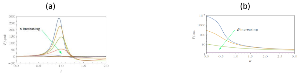
Figure 2: (a) Variation of peak contact pressure versus nondimensional time for values of \kappa = 0, 0.10, 0.25, \text{ and } 0.50 . (b) Variation of peak pressure versus \kappa for values of \beta = 0.001, 0.01, 0.1, 1, \text{ and } 10 .
