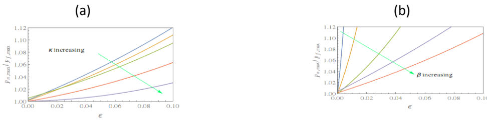
Figure 3: Nondimensional pressure variation as a function of protuberance height, \epsilon as a function of (a) \kappa (with values of \kappa = 0, 0.10, 0.25, \text{ and } 0.50 ), and (b) \beta (with values of \beta = 0.001, 0.01, 0.1, 1, \text{ and } 10 ).
